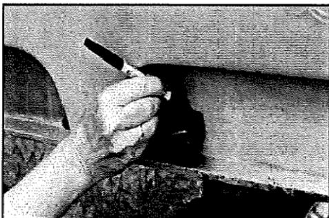
Photograph 2: Marking outline of hinge base on hull
